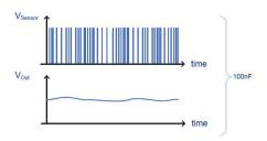
average analog value. For the resistive divider  $R_1$ =5M and  $R_2$ =100k .. 1M could be chosen.
